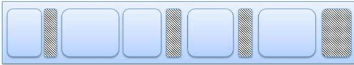
Fragmented memory before compaction
